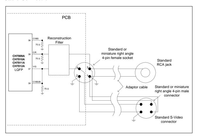
**Recommandation:** Please refer to Digi-Key or JAMECO for the standard socket & connector. Customer should be aware and consult the cable manufacturer regarding the EMI issue, when the small form factor custom made connectors & cables are required.
